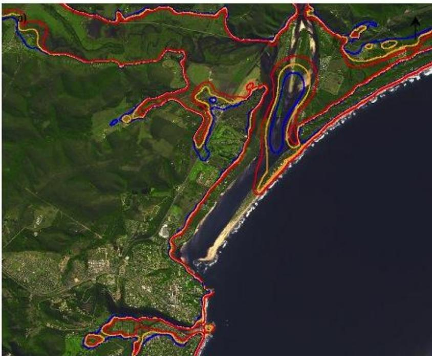
2.5 mamsl (red), 4.5 mamsl (orange) and 6.5 mamsl (blue) swash and flood contour lines for Piesang and Keurbooms-Bitou Estuaries (from SW to NE in a)). b) shows the current protective effect of undeveloped portions of the vegetated foredune at Plettenberg Bay.
